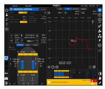
Firstly, an advanced, high-performance, and BV-certified DYNAPOS AM/AT & TCS dynamic positioning system, as well as an autopilot.
